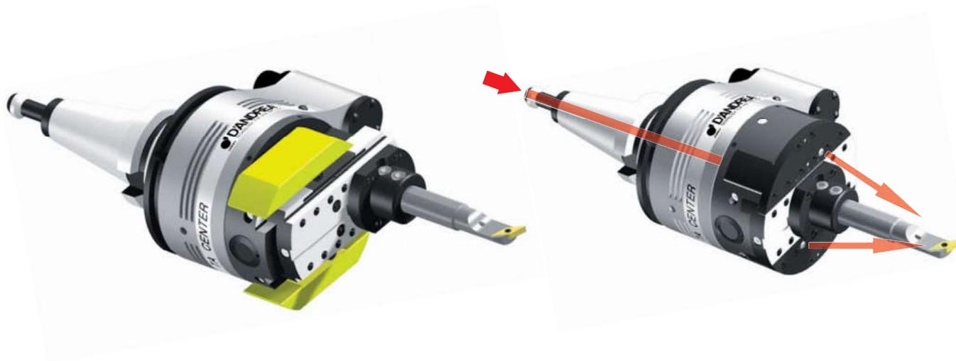
**GB** TA-CENTER heads are designed with two counter-weights for automatic balancing, that move opposite to the slide. Coolant exits from the two adjustable nozzles in the TA-CENTER located next to the slide after crossing the taper and the rotating body of the head.
