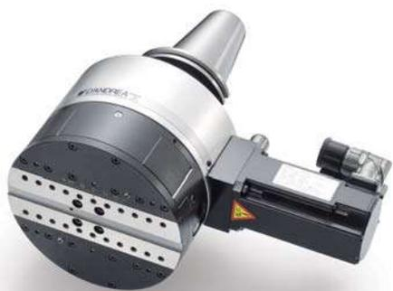
**GB** TA-Tronic boring and facing heads can be manually or automatically applied on small boring machines, machining centres and special machines. Connection with the machine tool spindle occurs through a cone for the rotation of the rotating head and a flange for fastening the fixed body on to the fixed part of the machine. For lighter tasks a simple anti-rotation pin may be used.
