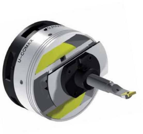
**GB** U-COMAX heads are designed with two counter-weights for automatic balancing, which move opposite to the slide making it possible to machine at a higher number of rpm without noticeable oscillations.
